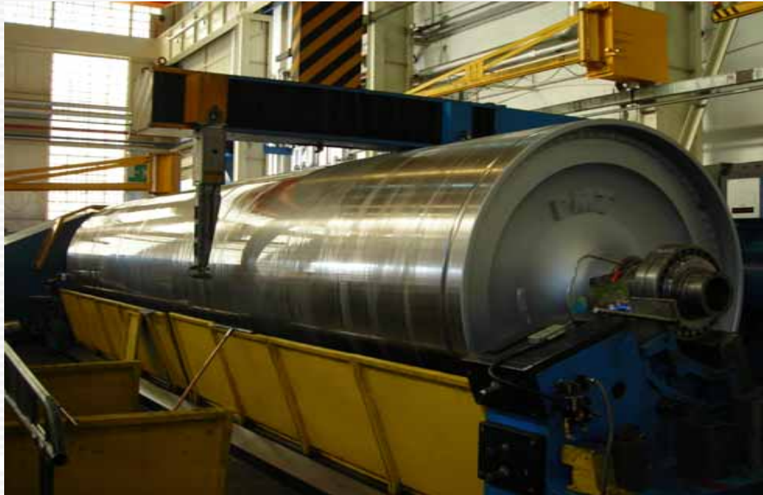
6' Paper Dryer being machined
